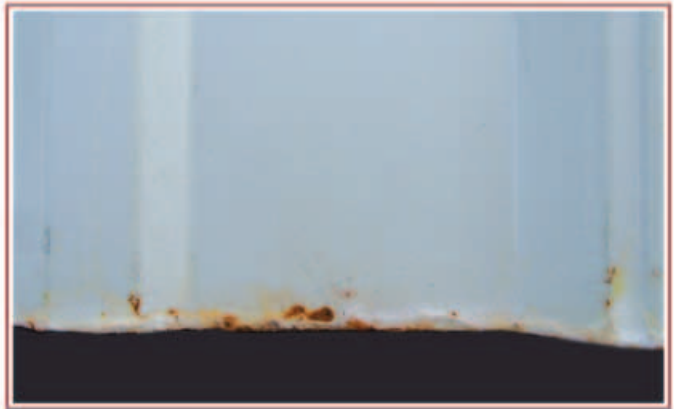
Overview of an Everlast II® panel without CECI™ exposed to 48 weeks of salt spray testing at 45° South Florida
