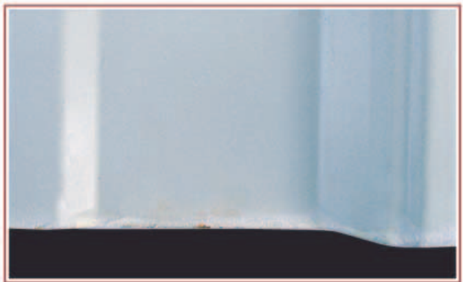
Overview of an Everlast II® panel with CECI™ exposed to 48 weeks of salt spray testing at 45° South Florida
