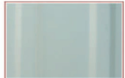
Overview of an Everlast II® OMNI panel exposed to 1,500 hours of accelerated acid rain testing
